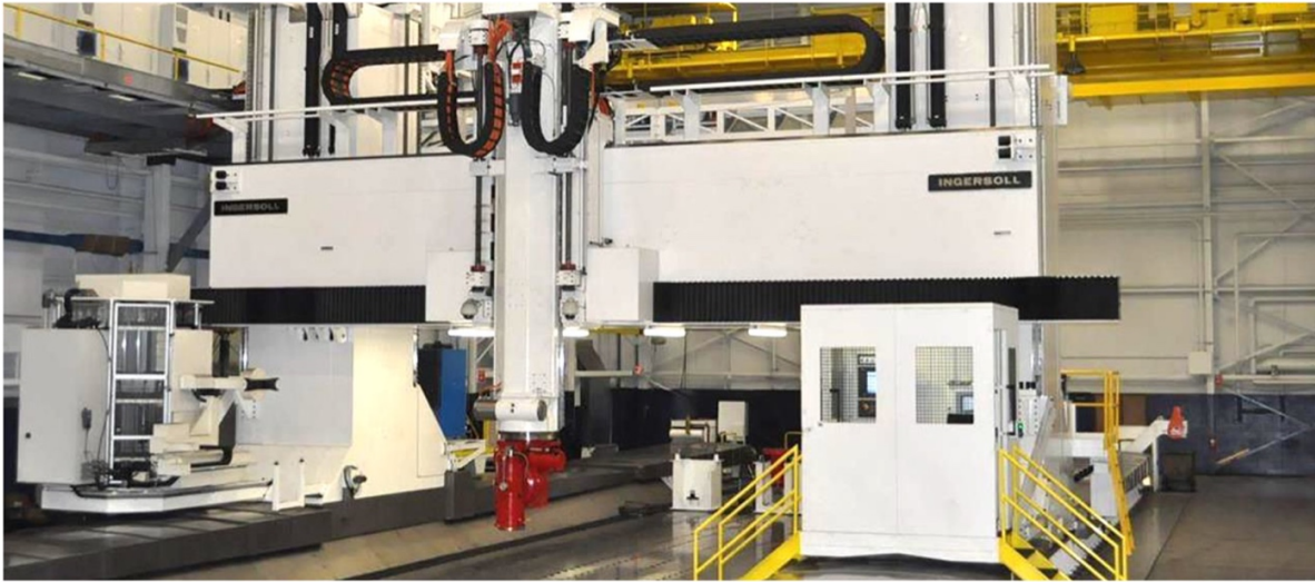
Figure 1: A gantry-type, large milling center
