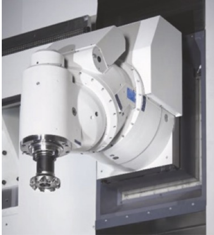
Figure 9: Universal milling head
