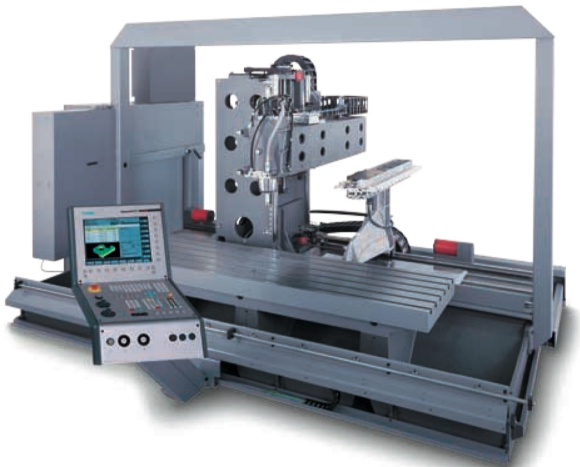
Figure 13: Travelling column machine
